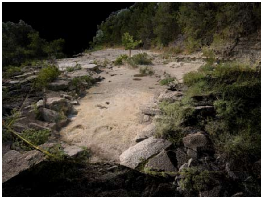
Figure 2. LiDAR scan of the main tracksite at Glen Rose. The image shows raw point cloud data, in which points have been colour-coded using images from the integrated digital camera.
