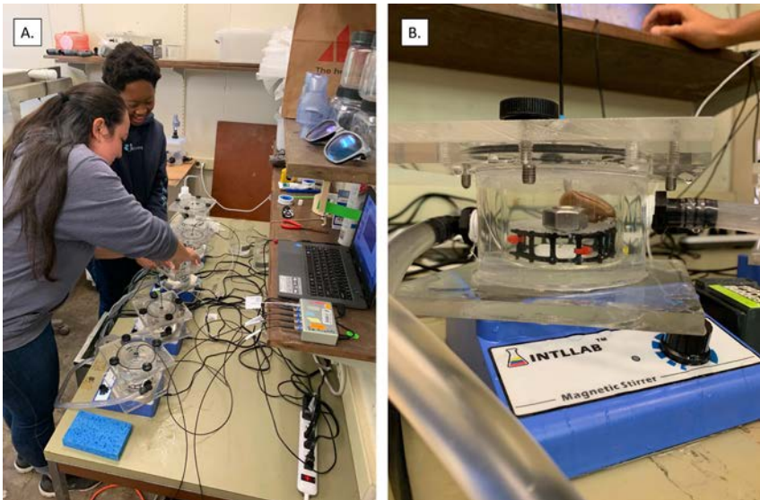
Figure 1. A) Stanford researchers Kyra Anderson and Kemi Ashing-Giwa set up experimental respirometry chambers for brachiopods at the University of Washington Friday Harbor Laboratories, USA. B) Close-up of experimental chamber. The chamber has a double-hulled construction, allowing temperature-controlled water to circulate through the middle volume. The internal chamber (holding articulate brachiopod Terebratalia transversa ) has a false floor with a stir bar underneath to enable water mixing. Standard metabolic rate and the minimum oxygen level required to maintain standard metabolic rate were measured for multiple individuals at multiple temperatures, allowing us to compare physiological traits between extant members of the Paleozoic and Modern faunas.
